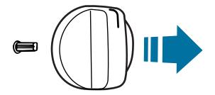
Loosen the locking screws inside the control knob.
